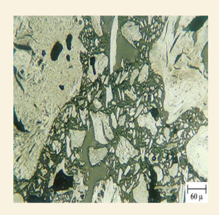
Graphite electrodes are made from two components: petroleum coke and coal tar pitch.
