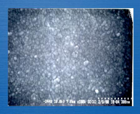
The non-aligned surface features correlate with the low degree of graphitization obtained at this temperature.
